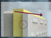
7. Edging sloped towards outer leaf to ensure wall ties sloped down.
