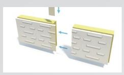
13 This pattern should be repeated with subsequent lifts repeating the position of the first board. Alternate boards should be cut to different lengths to create a brick bonded pattern if the corner boards have not been used.
